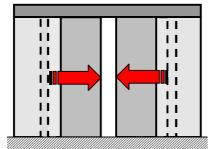
• Slide the door by hand to the closed position
